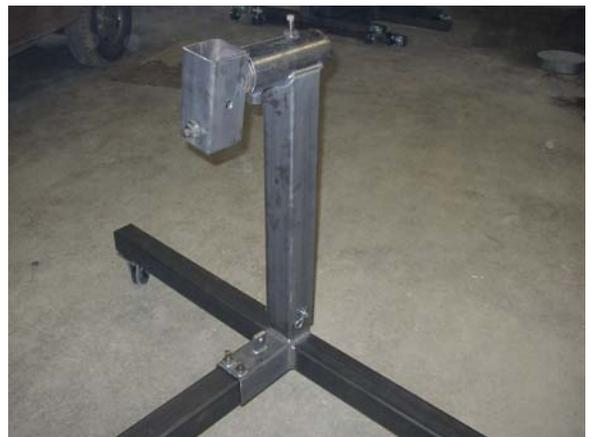
Install the hydraulic cylinder by passing the 5/8 x 2-1/2 bolt through the clevis on the bottom of the cylinder and the bracket on the base socket. Tighten the nut securely. Slowly pump up the cylinder and guide the shaft into the socket on the bottom of the large pivot tube. Align the holes at the bottom and insert the hitch pin.
