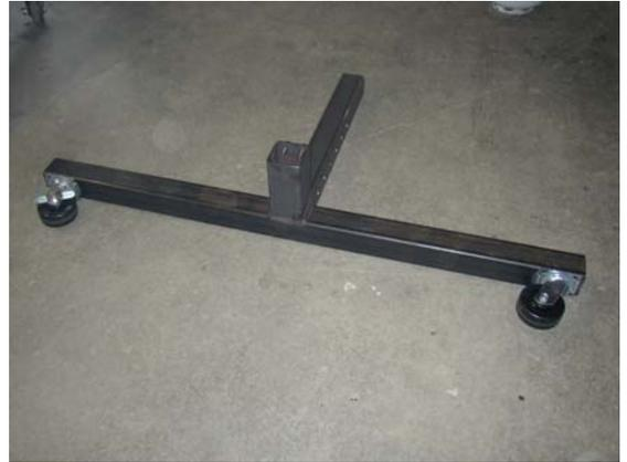
Insert the base unit with the single caster into the socket and tighten the two set bolts securely. Grease all the zerks on the casters. There is a zerk on both the axle and the turntable.
