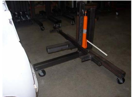
Set the attach brackets at the same distance center to center as the holes you will be using to secure the car body to the CAROTATOR. Be sure you position the attach brackets the same distance either side of the center of the horizontal support arm.
