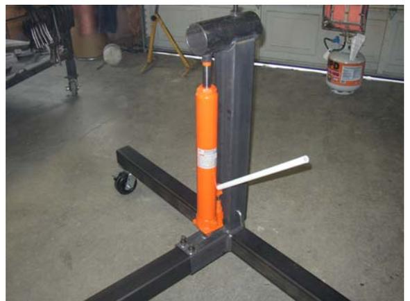
Install the support arm into the pivot bracket socket and secure with the hitch pin.
