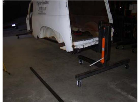
Repeat the above on the other end of the car. You can insert the center bar into the second half as shown at this time and mate it to the other CAROTATOR half as you place the second half as shown here, or wait until last to install the center bar.
