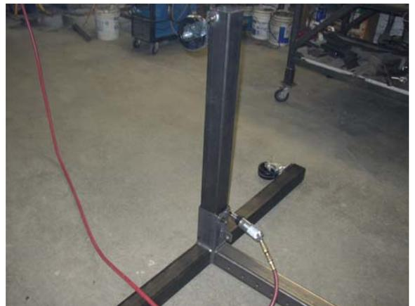
Right the unit onto the casters. Grease the “male” pillar liberally by pumping grease onto it and smearing it all over with a rag. Slide the large “female” pillar / pivot assembly onto the vertical “male” pillar. Grease the pivot by removing the set bolt and pumping about 20 pumps through the square nut.
