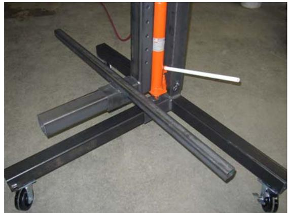
These photos show both units together with the center bar and the center bar coupling socket. If you picked up your CAROTATOR, the center bar will be in one piece and there will not be a coupling socket. Normally you will not assemble the center bar until assembling the car on the CAROTATOR.
