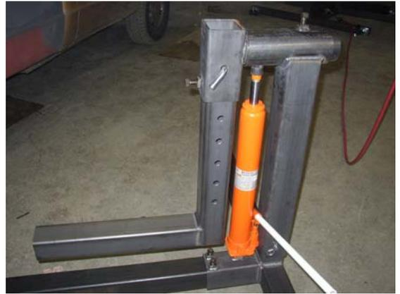
Slide the support cross member onto the horizontal member of the support arm. Repeat for the other end unit.
