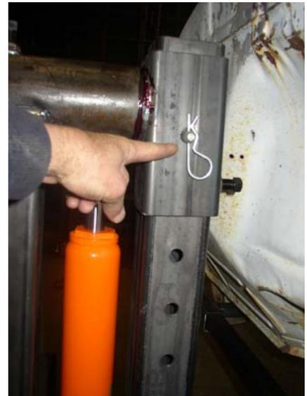
Once you have the car body balanced, it is necessary to raise the pillar to allow enough vertical clearance to rotate the carbody 360 degrees. (See middle photo)
