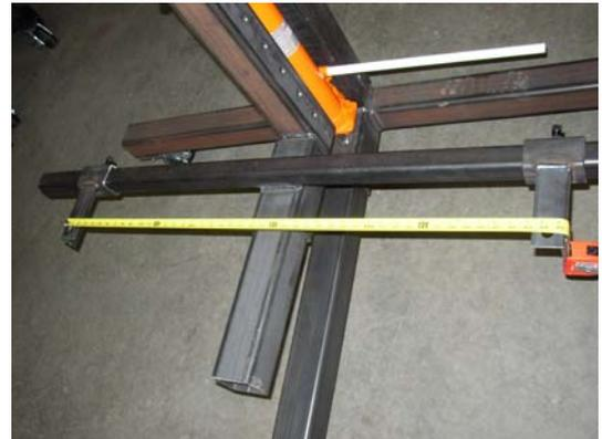
Once the attach brackets are properly spaced, roll the CAROTATOR unit underneath the car and raise it using the hydraulic ram to mate with the body. Using a small block of wood or plywood between the attach bracket and the car body will give a better grip and prevent slipping and creaking as you rotate the body.
